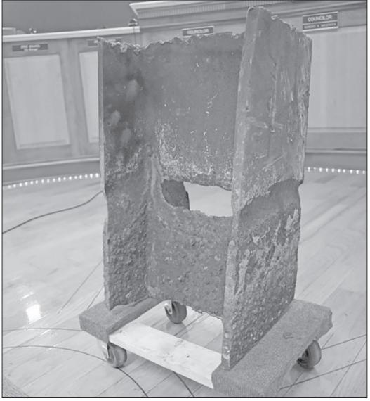
A corroded H-pile, part of the structural foundation for the **Lakeshore Drive** parking deck, sits in the Houghton City Council chambers Wednesday night. Houghton City Manager Eric Waara presented the piece as a visual example of the decay observed in a U.P. **Engineers & Ar**chitects report on the deck. (Houghton Daily Mining Gazette photo)
