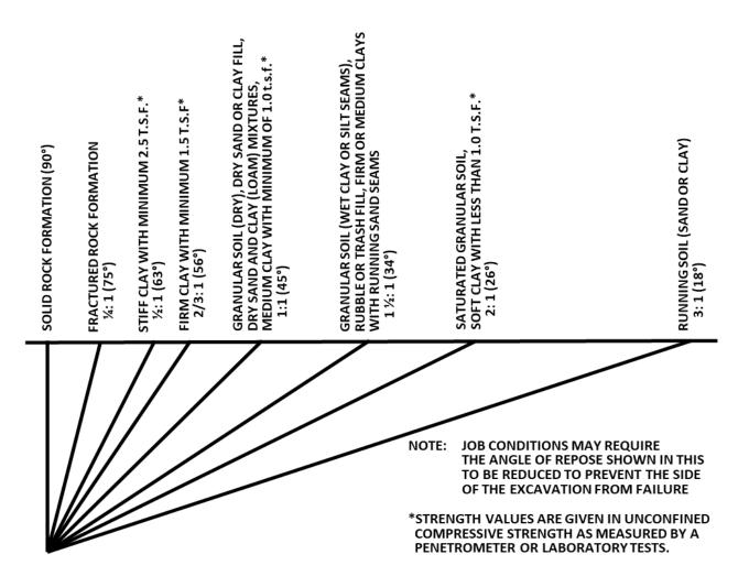
R 408.40942 Supporting systems; angle of repose; tie backs; sheeting; additional bracing.
